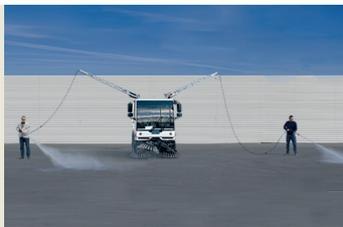
**Boom with reel and hand lance** Two booms are mounted on the hopper with a reel and a hand lance that are connected to the highpressure water system of the CityCat 5006. These are useful for flushing rubbish from the sides of the street directly in front of the sweeper to significantly increase the working width and efficiency.
