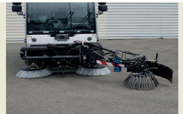
**Road construction brush** The robust brush is particularly suited for heavy use on road construction sites and weed removal applications. It provides a large working area and even better coverage in curves. Furthermore, it has a ground pressure control and a bidirectional tilt adjustment.
