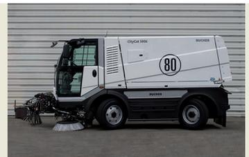
**Speed 80 km/h** The 5 m<sup>3</sup> compact CityCat 5006 street sweeper is also available in an 80 km/h variant. This allows it to travel and sweep on motorways and other fast stretches of road.
